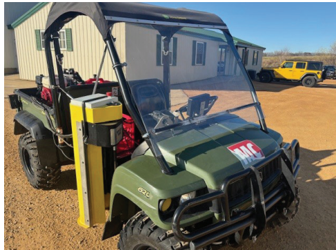
Soil Sampler: Mid-County Coop's soil sampling equipment takes consistent and accurate cores from the field.
